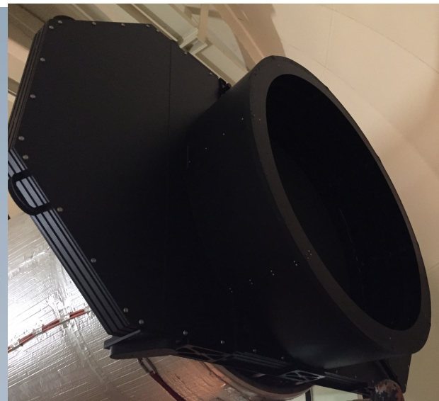
new Bonn shutter mounted on P48; new drive motors
